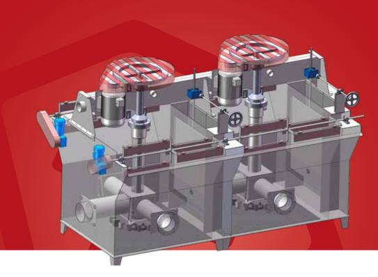
SUB-A type flotation cells, acknowledged as a classic worldwide, have been manufactured by Tüfekçioğlu for more than a half century.
