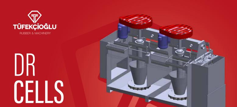
DR cells, developed after SUB-A cells, are open-flow type (the pulp flows freely from cell to cell through an opening at the bottom of the cell), with a bucket shaped container over the impellers of each cell that enables proper mixing. They are used especially in the flotation of finely ground base metal ores and lower density industrial raw materials with relatively larger sizes and coal.
